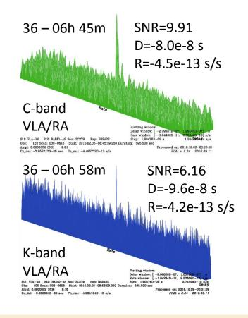
3C279 fringe detection on 18.5 ED (235000km) baseline at 22 GHz: 12μas fringe spacing!
