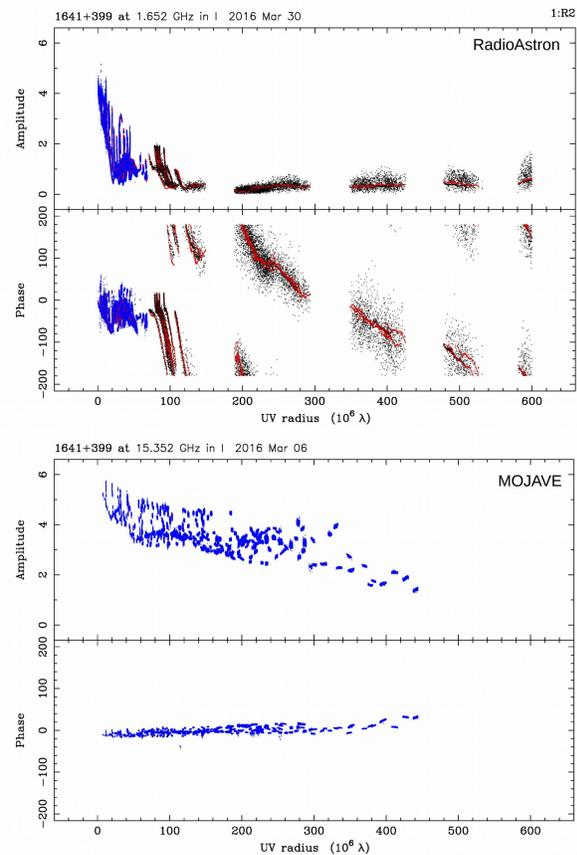
*Top:* Visibility Amplitude and phase as a function of UV radius for 3C 345. *Upper panel:* L-band data with RadioAstron. The black data points correspond to the space baselines, red shows the source model (blue contours in the figure at the bottom panel in the left hand side of the poster); *lower panel:* At 15 GHz observed with the VLBA in the MOJAVE survey (see Lister et al., 2009, 2018) at March 5<sup>th</sup>, 2016. The RadioAstron data show more extended structure.
