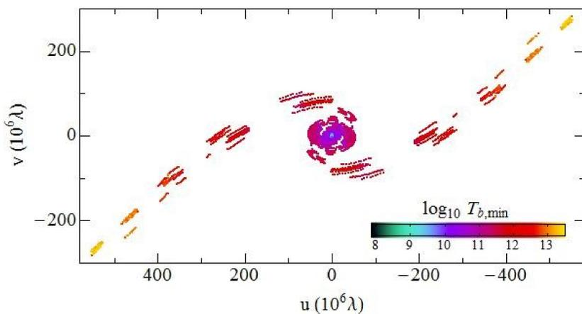
*Top:* UV coverage with RadioAstron, with the color scale indicating the minimum brightness temperature inferred from the visibility amplitudes (Lobanov 2015). These measurements imply a brightness temperature in excess of  $3.4 \times 10^{13}$  Kelvin in the most compact regions of the jet.
